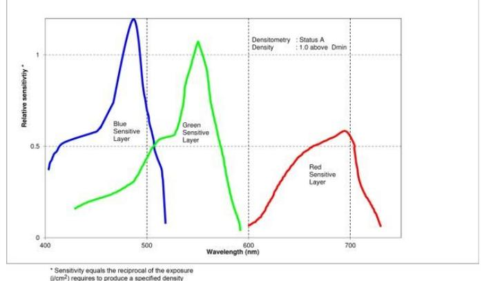
\* Sensitivity equals the reciprocal of the exposure (J/cm<sup>2</sup>) required to produce a specified density
